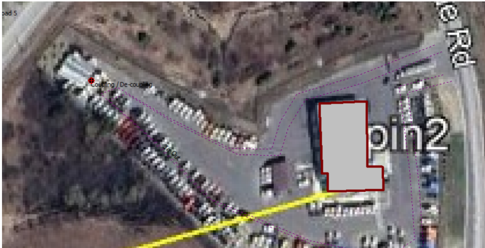
Figure 5 - Noise Model set up - Location of the significant noise sources – Impulse noise coupling and decoupling
