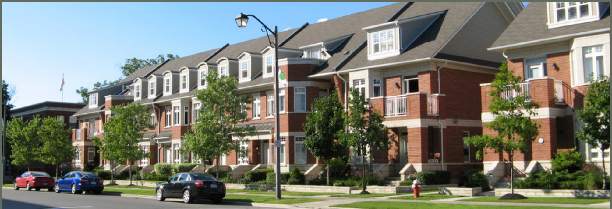
Image example of a front-loaded townhouse block with façade articulation that provides variety along the streetscape.
