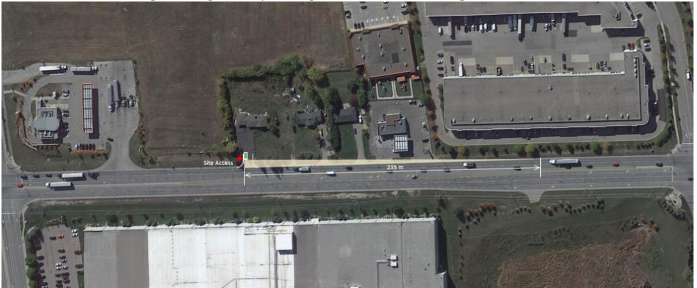
Figure 13: Single Unit Departure Sight Distance - Site Access at Regional Road 25
